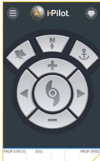
The buttons are deactivated when the app is not connected to a motor.
