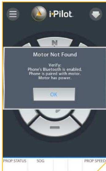
The "Motor Not Found" screen will appear when the app launches and the motor is either not powered up, connected with Bluetooth or paired to the device.
